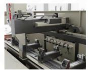
Double-Linear Guide bridge systems have are more rigid and durable compared to single-Linear Guide bridge systems. Reduced vibration and allows for more precise processing of the profiles.
