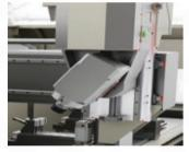
By focusing on providing convenient solutions for customers, and combining power and precision, GARNET XS4 lets the processing capacity be only limited by the users imagination, thanks to the 5.6 kW spindle motor with automatic tool replacement feature.
