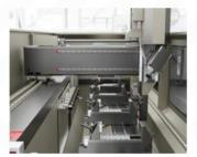
Thanks to its built-in automatic magazine with capacity for 8 tools, GARNET XS4 saves time when switching to different operations.The GARNET XS4, which positions its clamps ful-ly automatically using the X-axis, completely takes on the user's
