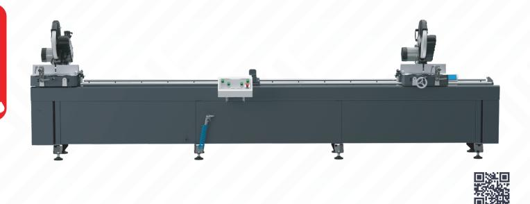
The GEMINI – II M, a manual, button-controlled double-head cutting machine with a 400 mm saw, is ideal for cutting aluminum, PVC, and wood profiles at various angles and thicknesses. The GEMINI – II M provides manual, fast positioning thanks to its X-axis control with a handwheel and ruler, while delivering a perfect cutting process. The GEMINI – II M, with its automatic horizontal and vertical clamps and profile support unit, enhances cutting quality while prioritizing its economic feature.
