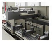
Double-Linear Guide bridge systems have are more rigid and durable compared to single-Linear Guide bridge systems. Reduced vibration and allows for more precise processing of the profiles.
