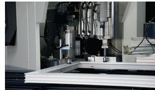
11 pieces of profile cleaning blade and two independend cleaning unit, cleaning bottom, top, interior and external surfaces of the profile.
