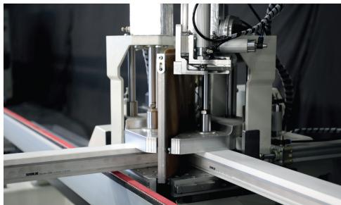
Through its electronic thermostat heat adjustment between 0°C - 350°C, welding time adjustment and digital controlled heat, quadruple welding unit provides scattering homogenised to plaque of heat.
